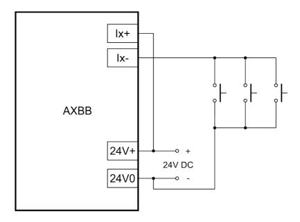
The other way is to connect the positive power supply rail 24V to one side of the NO switch and connect the other side of the NO switch to the positive input screw terminal of the AXBB-E and connect the 0Volts (24V0) to the negative input screw terminal of the AXBB-E.
