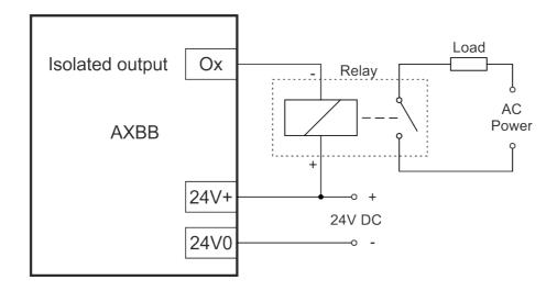
9.1.2 .Connecting a solid state relay (SSR)
