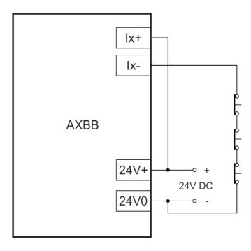
The other way is to connect the positive power supply rail +24V to one side of the NC switch and connect the other side of the NC switch to the positive input screw terminal of the AXBB-E and connect the 0V (24V0) to the negative input screw terminal of the AXBB-E. The following image shows the connection:
