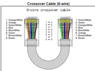
Use this cable for connection via router(s).
