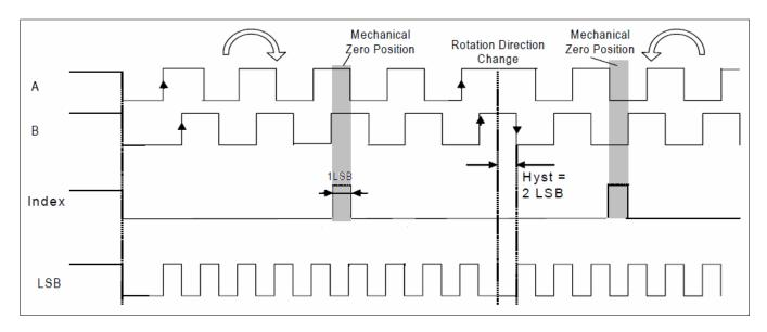
To avoid the flickering of the encoder signals a 2 counts (LSB) length of hysteresis is introduced.
