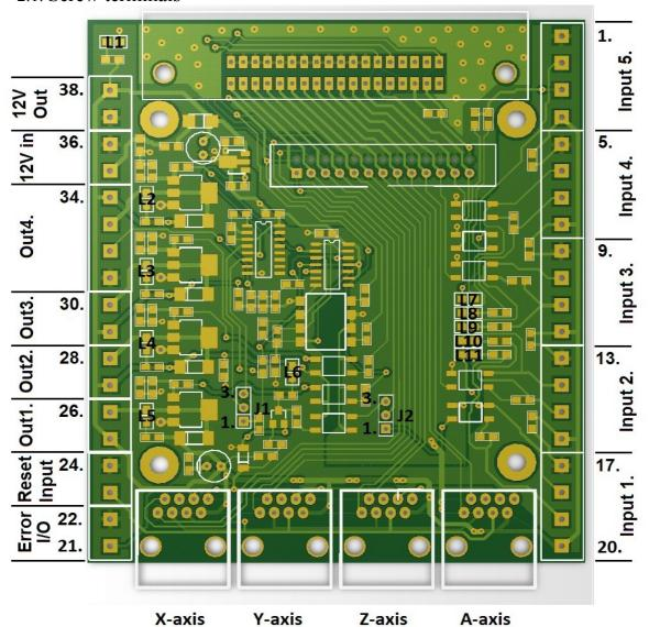
Screw terminals have standard RM5.0 pitch and connections of external devices can be made through these connectors.
