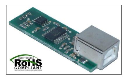
The USB programming stick (PRG01) is used to connect our DG2S servo drives to the host PC for configuration and for making diagnostics.
