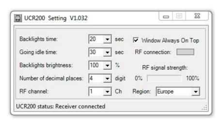
Moreover on this screen informations also shown about the RF signal actual strength and if the device established a vital connection with it's receiver.
