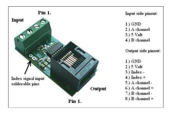
The differential line driver can be used to convert single ended to differential signals.
